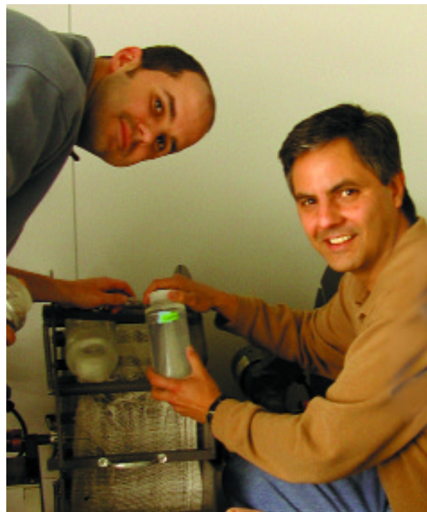
Hans Dam, right, and Sean Colin, left, put samples into a "plankton wheel". Like a miniature ferris wheel, this equipment simulates the natural conditions in which plankton move with the flow of water.
