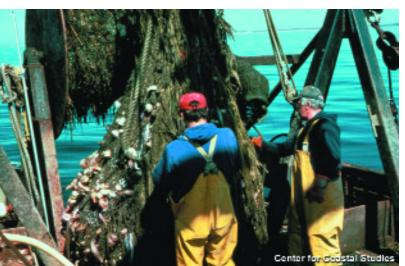
This commercial fishing vessel uses trawl nets, one of many types of fishing gear operated in the coastal waters of the U.S. These nets sweep across the bottom, held open by "doors" on each side of the net.
