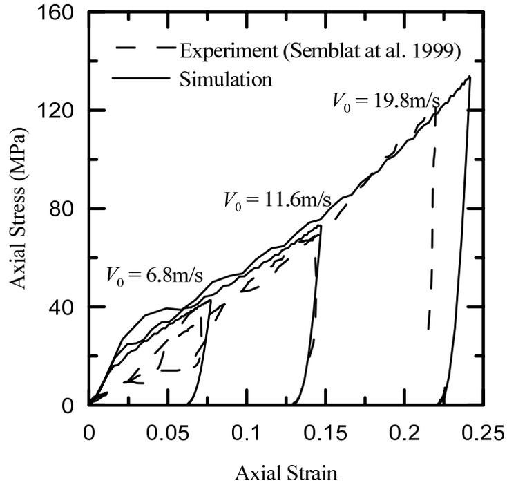
Figure 6. Axial stress versus axial strain of Fontainebleau sand in split Hopkinson pressure bar tests
