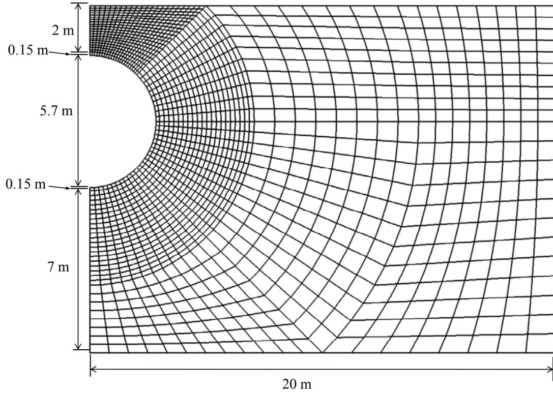
Figure 7. A typical finite element mesh used in the analysis of tunnels (the tunnel center line is at a depth of 5 m below the ground surface)
