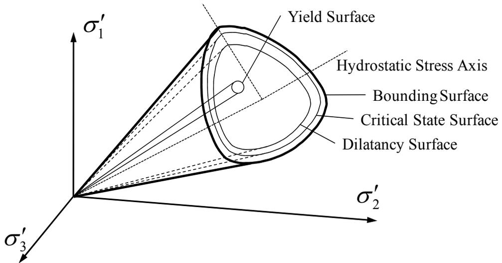
Figure 2. Model surfaces in three dimensional stress space
