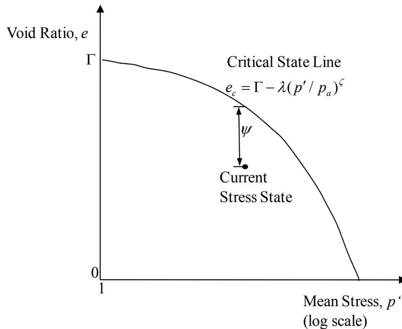
Figure 1. Critical-state line and state parameter
