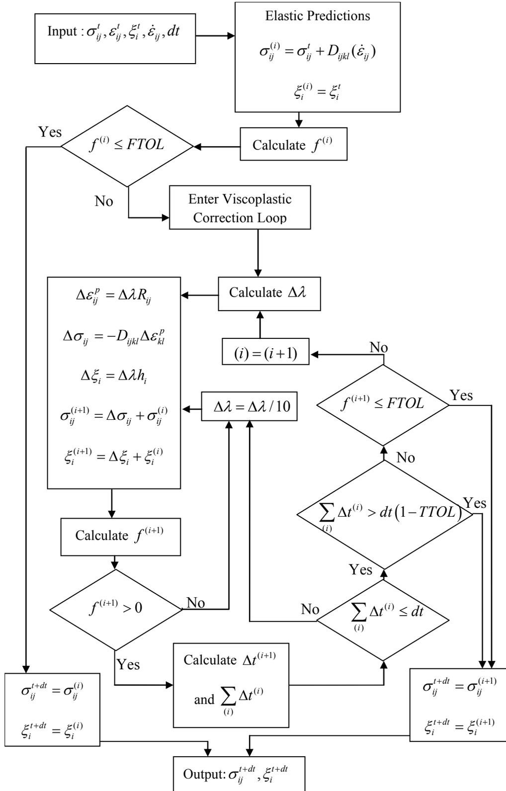
Figure 3. Cutting plane algorithm flow chart
