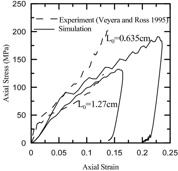
Figure 5. Axial stress versus axial strain of Ottawa sand in split Hopkinson pressure bar tests
