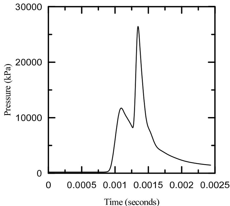
Figure 9. Pressure amplitude curve for the explosive C4 of radius 0.1 m in a tunnel with an internal radius of 2.85 m
