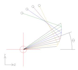
FIG. 2: A simplified drawing of how the HTCC works. The four colored curves are each a section of one of the four ellipses from figure 1. Mirror 1 is shown in green and occupies from
