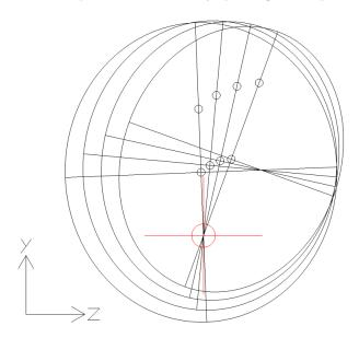
FIG.1: The four ellipses. The origin of the absolute coordinate system is indicated in red. The eight smaller circles indicate the positions of the ellipses' centers and focal points. All of the ellipses share a common focal point at the origin. Also shown are the major and minor axes of each ellipse.
