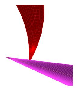
FIG. 15: The cone used to cut the bottom of mirror 4. Its axis of symmetry lies on the z-axis and its surface forms an angle of  $5^{\circ}$  with said axis. The tip of the cone is at the origin of the absolute coordinate system.
