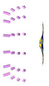
FIG. 17: A side view of the HTCC mirrors and PMTs.
