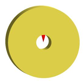
FIG. 14: The cylindrical shell used to cut the top of mirror 1. Its inner radius is 1165.5073 mm, it's outter radius is chosen such that it is large enough to cut away the unwanted part of the mirror, 5500 mm was chosen.
