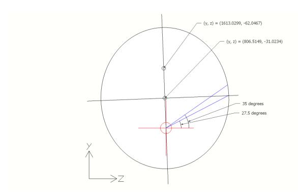
FIG. 6: The ellipse defining the front surface of the mirror. The red lines show the origin of the absolute coordinate system. The ellipsoid is an ellipsoid of rotation and is created by rotating the ellipse about it major axis (y'). Shown in blue are the angles at which Čerenkov light will hit this mirror (mirror 1), 27.5° - 35°. The y'-axis forms an angle of 2.2029° with the y-axis. The x'-axis crosses the x-axis at x = -20997.9801 mm.
