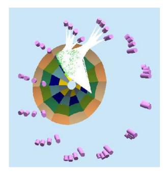
FIG. 18: Photons leaving the target follow the expected trajectory; they are reflected off of a mirror and hit the center of the face of the corresponding PMT.
