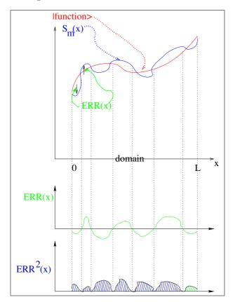
FIG. 1: Error involved in approximating a function.
