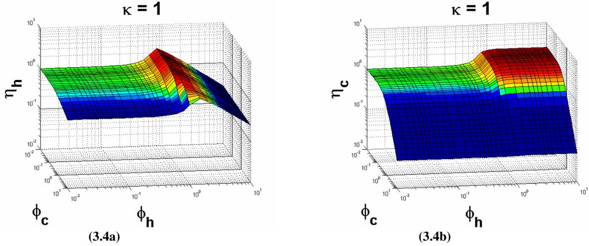
**Figure 3.4: Exothermic and endothermic effectiveness factors for a ceramic support wall  $\{\beta_h = 0.25,$
