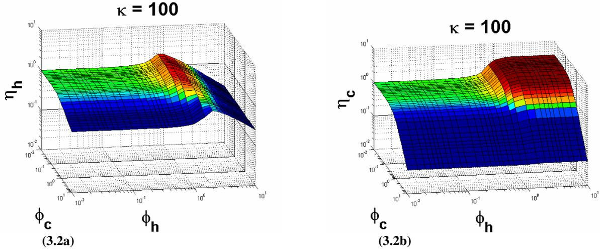
**Figure 3.2:** Values for the exothermic and endothermic catalyst layers for a steel support wall  $\{\beta_h = 0.25, \beta_c = -0.35, \gamma_h = \gamma_c = 20, \chi = 1, \kappa_h = \kappa_c = 100, Bi_{mh} = Bi_{hh} = Bi_{mc} = Bi_{hc} = 1000\}$ .
