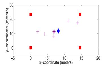
Fig. 9. Node deployment during March 2010 pool test. The transmitters are denoted by squares, and the receiver is denoted by the diamond. The scattered plus signs are the estimates by the exhaustive search method.
