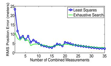
Fig. 11. Localization error during March 2010 pool test.
