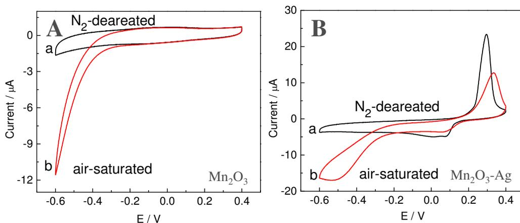
Figure 6. CVs of the (A)  $\text{Mn}_2\text{O}_3/\text{GCE}$  and (B)  $\text{Mn}_2\text{O}_3\text{-Ag}/\text{GCE}$  in  $\text{N}_2$  de-aerated (black) and air-saturated (red) 0.1 M pH 7 phosphate buffer solution at the scan rate of 100 mV/s.
