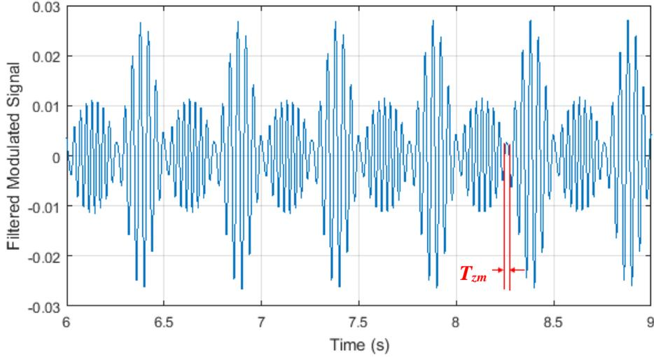
Fig. 4. The no-fault  $y_{pos}(t)$  signal for DE/ME with PFAM applied ( $\Delta f = 5$  Hz and  $f_p = 2$  Hz).  $T_{zm} = 24$  ms
