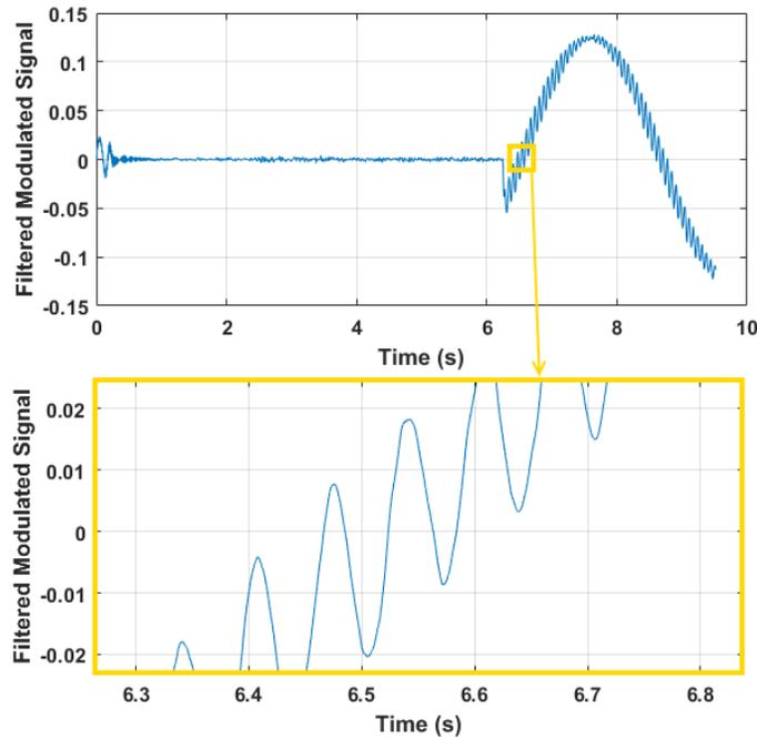
Fig. 6. Exemplary quick oscillations about zero after a PSH fault is injected at 6.2852s
